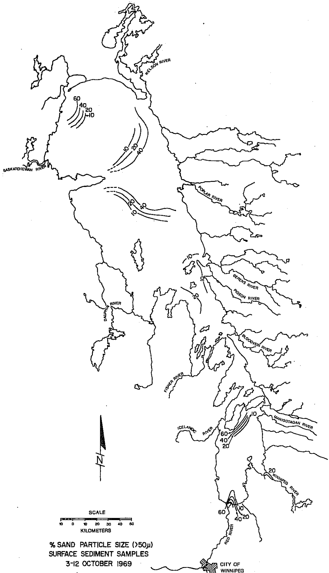
Fig. 8. Isopleths of % sand (2000-50 µm) in Lake Winnipeg sediments, based on Table 2 data.
